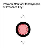
\*If the key is used as a presence key at the same time, the key must be pressed for at least 3s, in all other cases a short press is sufficient.
