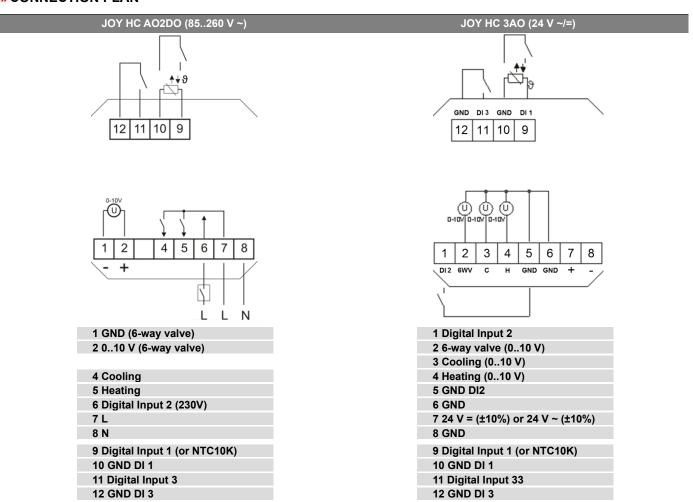
Note: Parallel connection of the potential-loaded inputs is not permitted!
