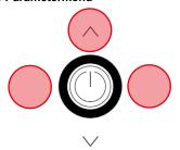
Access to Parametermenu: Press buttons for 3 seconds simultaneously
