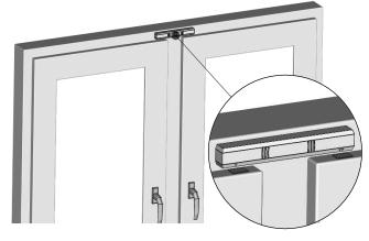
Mount the magnet flat as shown next to the arrow marking.
