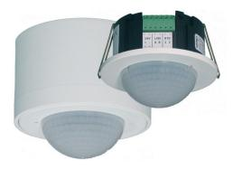
The LON multisensor lumina MS4 is a combination of occupancy sensor, two light sensors and infrared remote control receiver. An external temperature sensor can be connected.
