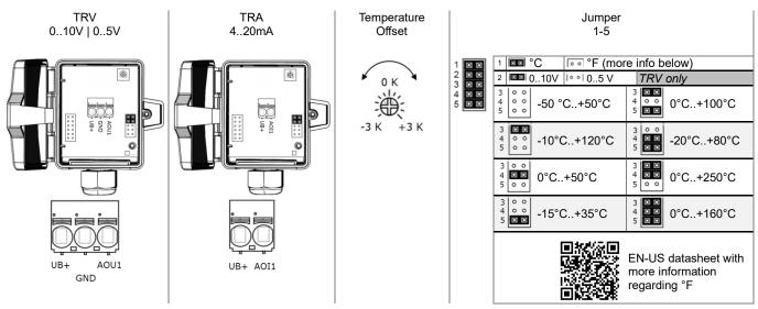
fig. (Measuring range and offset adjustment, default settings: -20 °C..+80 °C | 0 K)
