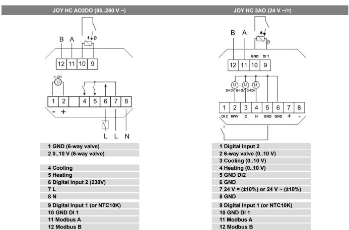
Note: Parallel connection of the potential-loaded inputs is not permitted!
