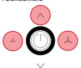
Access to Parametermenu: Press buttons for 3 seconds simultaneously
