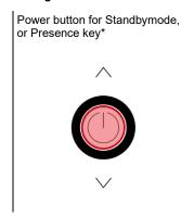
\*If the key is used as a presence key at the same time, the key must be pressed for at least 3s, in all other cases a short press is sufficient.
