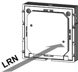
After delivery the room operating unit might be in default shipping mode, in this case press the learn button (<1 second) at the rear of the device [Signal telegramm will be send, SIG -> 0x0F // shipping mode deactivated].
