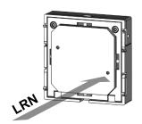
After delivery the room operating unit might be in default shipping mode, in this case press the learn button (<1 second) at the rear of the device [Signal telegramm will be send. SIG -> 0x0F // shipping mode deacticvated].
