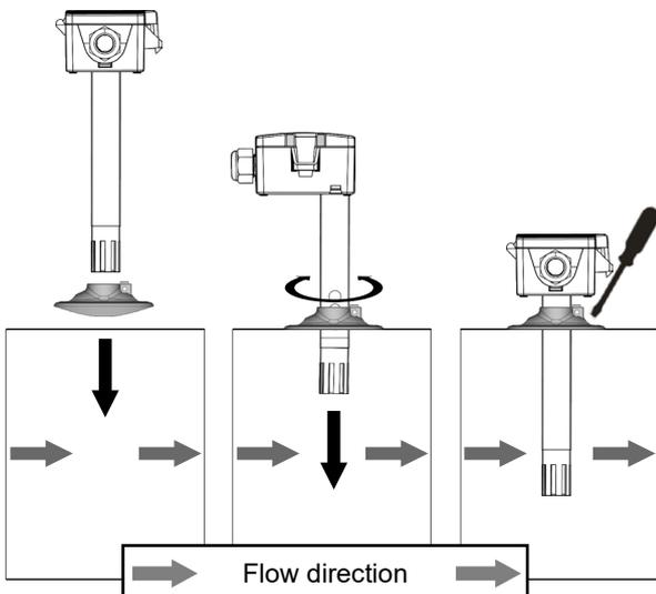
**Don't tilt the sensor during mounting / dismounting!**
